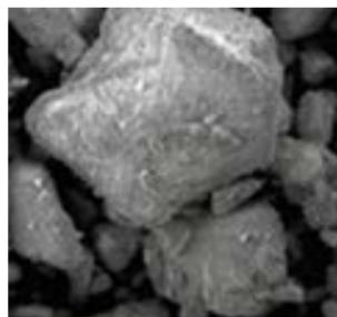
Particles with softened geometry (x1000)
