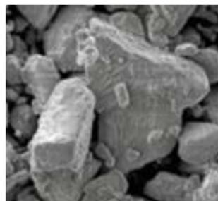
Stratified particles with aggressive geometry (x1000)
