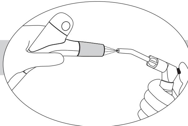
**⚠** The turbine connection and the connector must be absolutely dry. Moisture at the connection can cause blockage in the air/powder channels of the unit.
