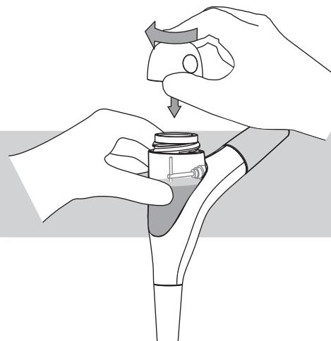
Clean the threads of the powder chamber before screwing on the cap.
