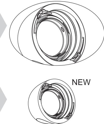
Check the state of the threads of the powder chamber and cap. The powder chamber is pressurized during use. The condition of the powder chamber and cap is an important safety factor.
