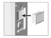
Push the filter in until the limit stop is reached.
