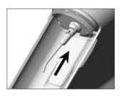
1 Insert the adaptor with the maintenance attachment facing downwards.
