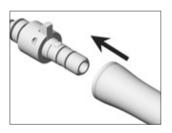
Push the transmission instrument onto the adaptor, with the coolant outlet facing downwards.
