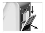
Remove the filter compartment cover.
