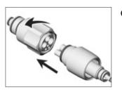
Push on the transmission instrument and/or adaptor on the Quick RM adaptor and tighten the union nut anti-clockwise by hand.
