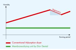
After longer operation of the compressors, moisture in the adsorption dryer increases. Yet the membrane dryer remains constantly dry and requires no interruption to supply.
